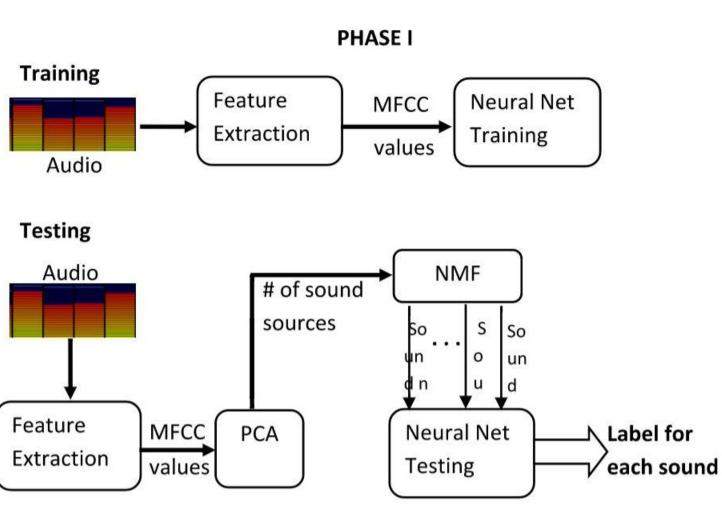
Training the Network: A Feed-Forward NN is used for sound event detection using labeled data. It is a 2 layered system.
