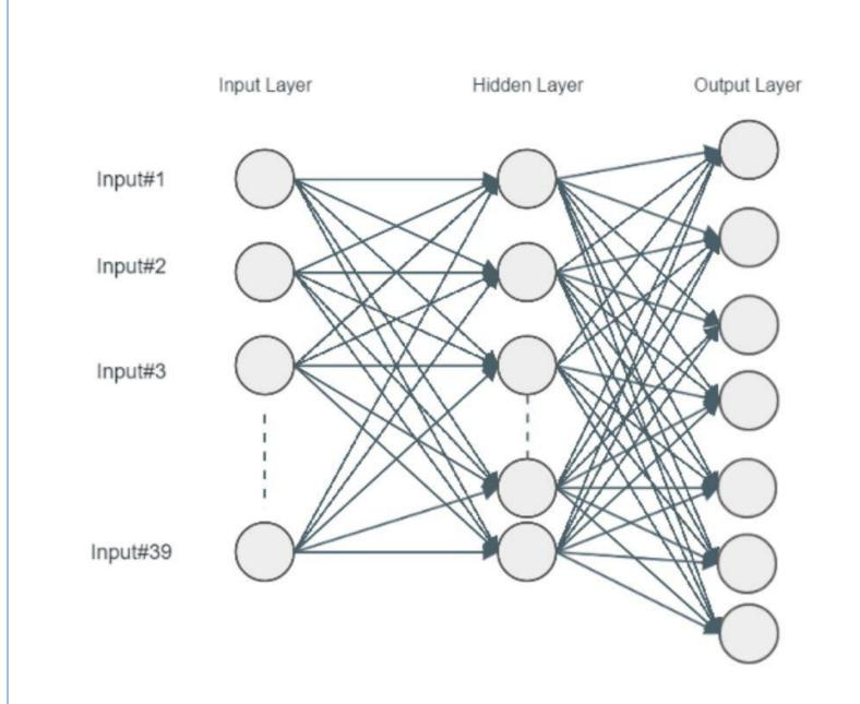
The NN hyper-parameters such as number of hidden units, mini batch size, learning rate and initial weight and bias etc. are selected by a grid search over the parameter values. The neural network was trained for 100 epochs with a mini batch size of 10, a learning rate of 3 and with an accuracy of average 70% (for correctly classifying sounds from the Urb\_data).
