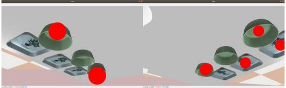
3) Integrating and modifying the grasp proposal logic (using a bounding box approach) -- grasp proposals are the possible poses that the robot arm can use to grab the object. Dense grasp proposal generation is a key component of ensuring that all objects are picked up. We integrated a grasp proposal approach based on Contact Graspnet and handled the corresponding coordinate transformations that followed leading to denser grasp proposals. We
