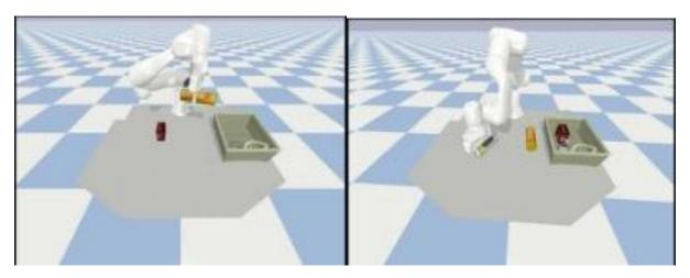
6) Experimenting between different simulators (PyBullet vs Sapien) -- Different simulators play a different role for different scenes as the underlying physics and object-arm interactions are different. We evaluated the performance of two simulators PyBullet and Sapien and all the tasks and optimized for the one with the higher accuracy (Sapien).
