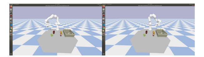
2) Handling duplicate objects by marking the objects already seen – The feature matching code provided in the baseline would fail in cases containing duplicate objects as it would assign a target pose to an already detected object. We added markers on already detected objects to prevent assigning multiple target poses to the same object.
